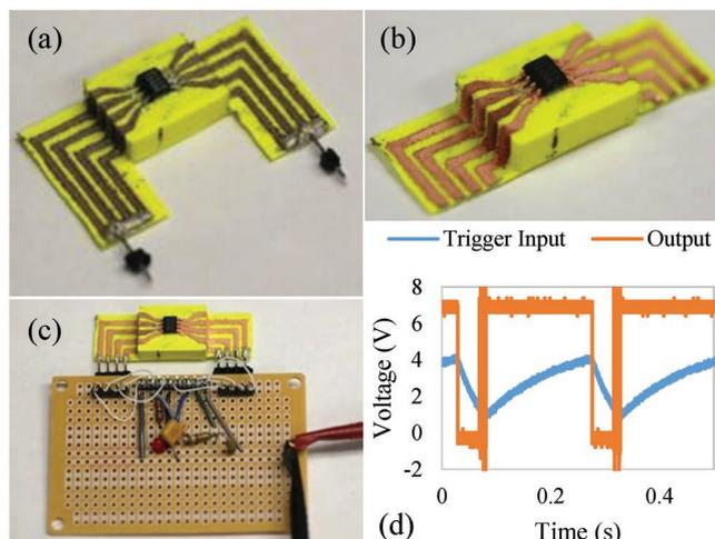
**Figure 3.** a) 3D printed SOIC8 mount with 555 timer chip, b) SOIC8 mount after plating and removal of breakaway region, c) astable 555 oscillator circuit, and d) circuit output.
