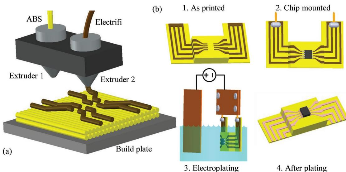
**Figure 1.** a) Dual extrusion fused filament fabrication and b) electroplating process.
