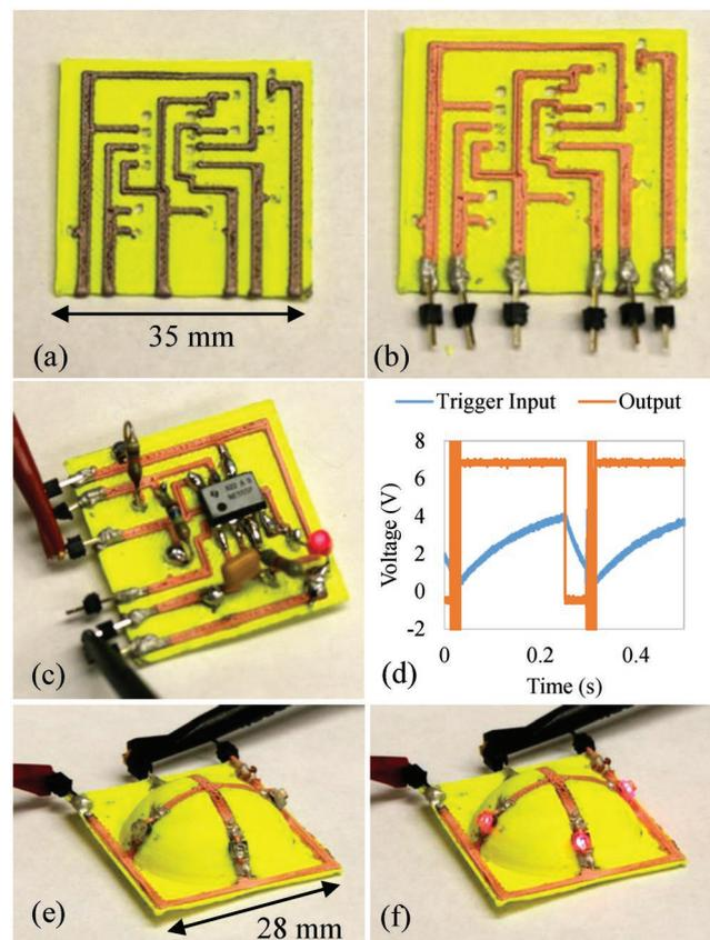
**Figure 4.** 3D printed astable 555 timer circuit a) as printed, b) after plating, c) tested after soldering, and d) circuit output, and plated traces connecting to LEDs on a hemisphere e) before and f) after LEDs turned on.
