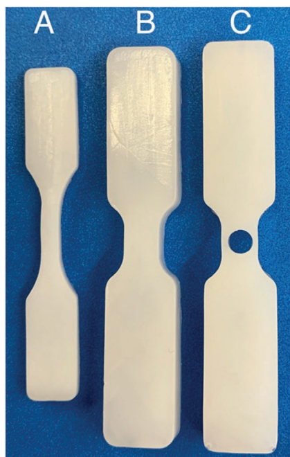
Figure 2. Representative optical images of PVA hydrogel samples: A) ASTM D638-14 Type V shape for monotonic tension, B) customized fatigue tension sample for a sharp edge crack, and C) customized fatigue tension sample for a cylindrical hole.
